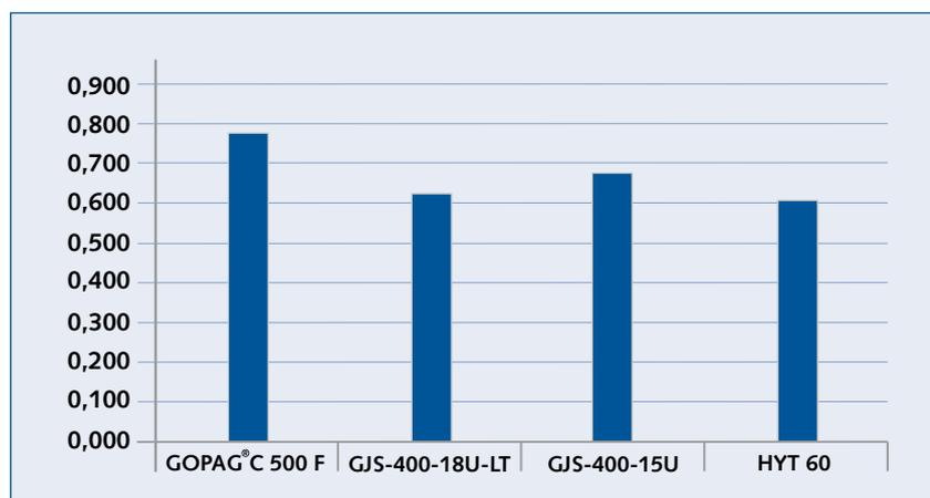
The yield strengths determined as the product of yield strength ratio and bursting pressure ( $R_{p0,2} / R \times P$  bursting pressure) (Fig. 5) show the
